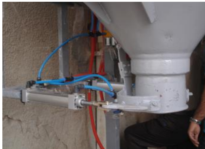
Figure 2: A photo of the mechanical bag holder, and the pneumatic valves/ pistons
